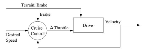
The internal state can be set by the input variable "brake" as well as by external commandos.
