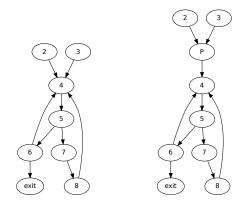
loop optimizations need CFG node before the loop to move code out of the loop
