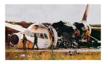
The failure was caused by adopting two unnecessary preconditions to landing (weight on wheels, wheels spinning). They were introduced because of an earlier accident (Lauda Air) where reverse thrust was applied during normal flight, wrongly assuming the plane was about to land.
