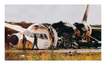
The failure was caused by adopting two unnecessary preconditions to landing (weight on wheels, wheels spinning). They were introduced because of an earlier accident (Lauda Air) where reverse thrust was applied during normal flight, wrongly assuming the plane was about to land.
