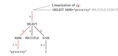
$c_{\mathbf{X}} = \{0, 1, 1.1, 2, 3, 3.1\}$  Failure occurs, reduce length
