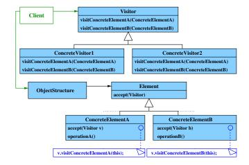
A concrete visitor (e.g. ConcreteVisitor1) wants to call operation operationA on ConcreteElementA elements and operation operationB on ConcreteElementB elements. Based on the class diagram shown above, provide a UML sequence diagram for applying the visitor to two elements, one of each class.
